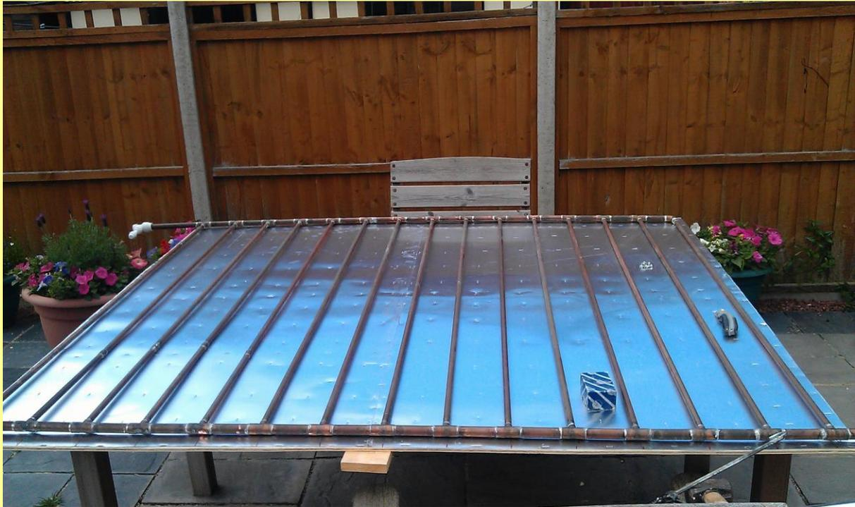
***I covered a 6mm piece of shutter ply with aluminium sheet using staples. Put the manifold on top and fastened the absorber plates on with staples and screws. I used screws because at this stage it had to be lifted vertically into my shed and staples on their own would not hold.***
