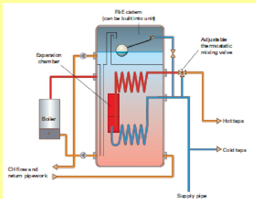
This type of system is open vented, so open to atmosphere on the primary side. The hot water is un-vent but because there is no volume of stored hot water it only needs to small expansion vessel to stop it expanding back down the main. The primary water is stored at 75°C so a blending valve is needed to cool the hot water down before going to my hot water appliances.
