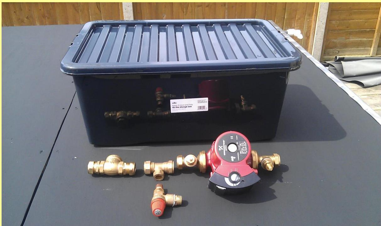
***I brought a five pound lining box big enough to accommodate a pump, isolating valves, pressure relief valve and a flap valve.***
